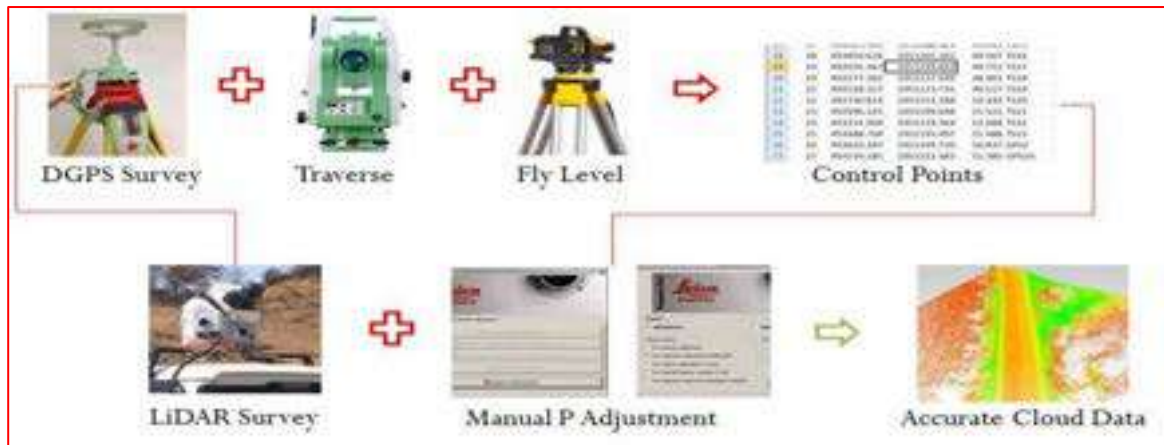
Figure 4.1: Process of Data Capture Work in field using Mobile LiDAR
