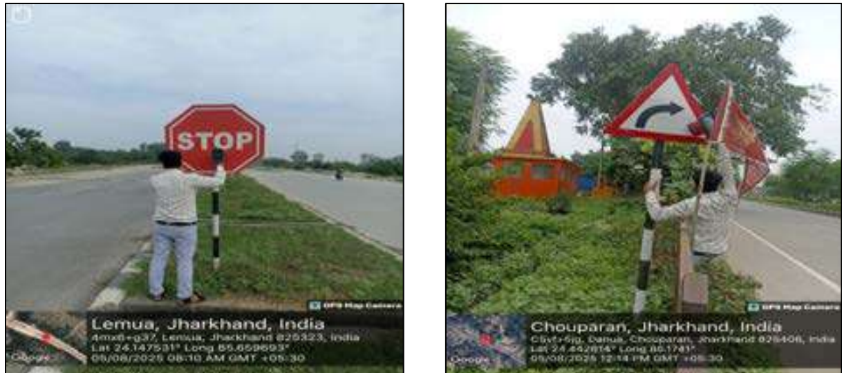
Figure 4.27: Retro-Reflectivity of Road Signs
