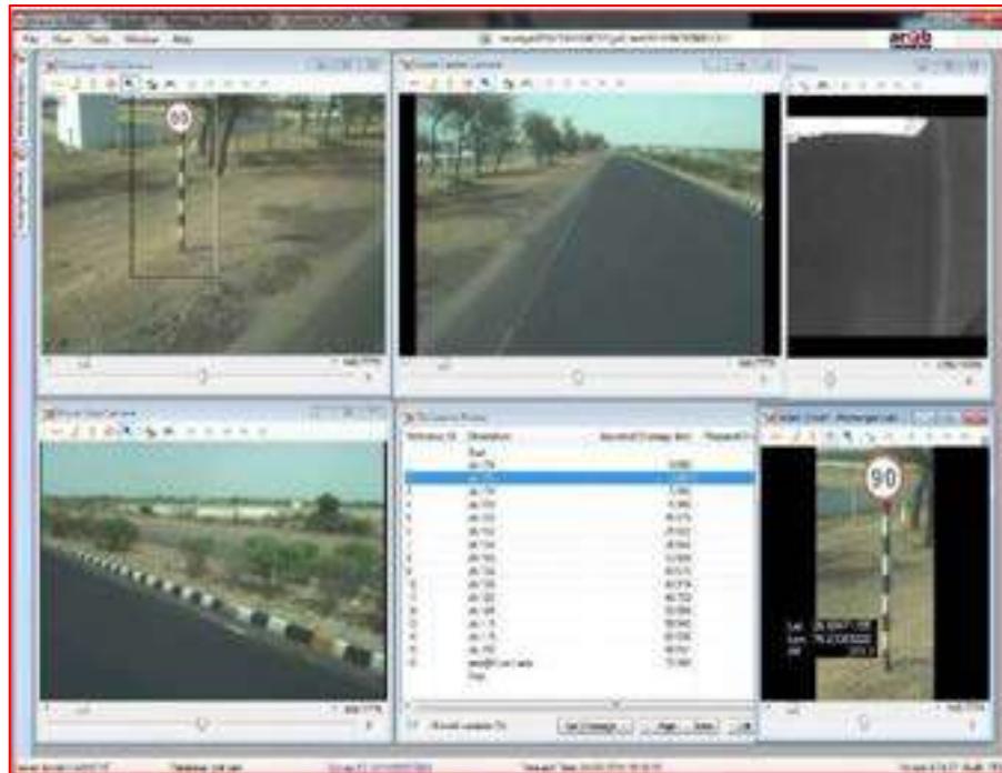
Figure 4.6: Roadside Furniture Location and Assessment
