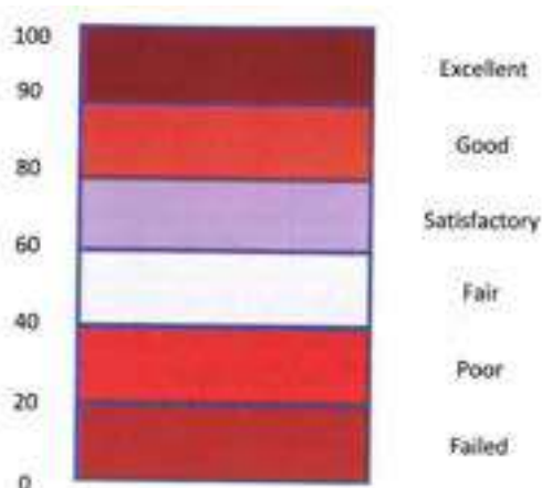
Figure 6.14: Pavement Condition Index
