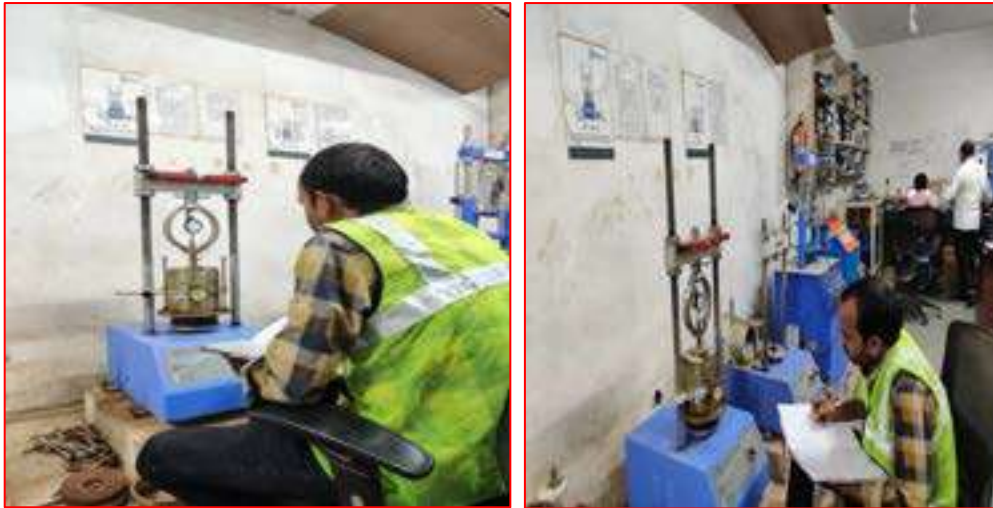
Figure 4.13: Days Soaked CBR Test
