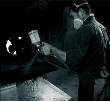
To ensure high-quality finish on our products, we use variety of techniques. We apply abrasive compounds and rotating buffs to create a smooth surface. Additionally, physical vapour deposition coating is applied to metals to enhance their durability, resistance to wear, and aesthetic appeal. Further, acrylic polyurethane and lacquer coats are used to protect the wood, and enhance its appearance.
