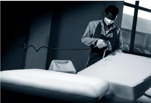
Foaming involves the application of foam materials for comfort and support. The process typically includes the integration of webbing and netting to ensure proper distribution and containment of the foam within the wooden frame. Webbing is used to create a supportive foundation, providing strength and stability to the seating area. Meanwhile, netting acts as a barrier, preventing the foam from shifting or sagging over time.
